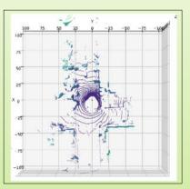
Bird-eye view of simulated lidar data.
