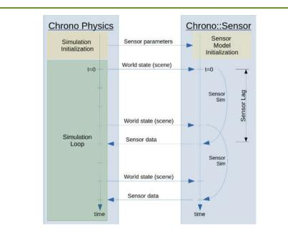
An illustration of the connection between Chrono and Chrono::Sensor shows the ability for dynamics to control the evolution of the environment. Data is generated with parameterized lag, update frequency, and sensor-specific models, and provided to the user for software-in-the-loop testing. Results from an example autonomous vehicle simulation using Chrono::Sensor
